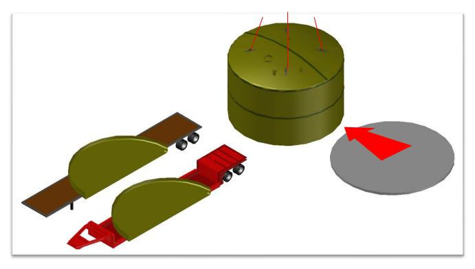
• The bottom halves are removed from the truck and placed on the pad with the use of a crane or telehandler.
